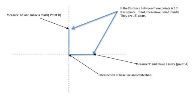
Once Point B has been established, the centerline is run from the intersection point through point B.
